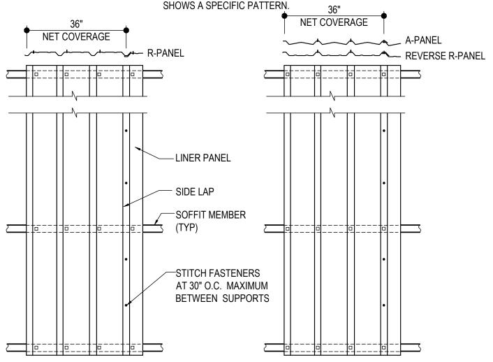
SOFFIT PANEL ERECTION DETAIL
